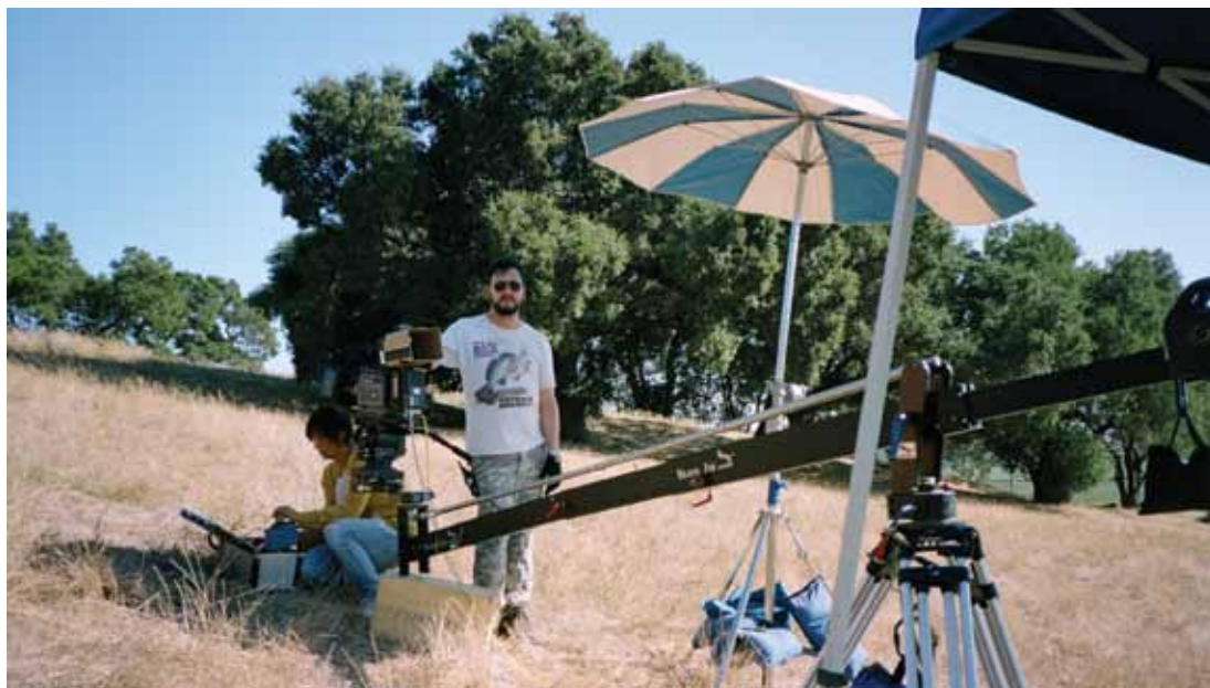
Meanwhile, Monika & Randy set up the establishing shot at the bottom of the hill. Here the F35 is mounted on a Panther Vario-Jib. We typically used an 18mm Leica Summilux-C lens for wides.
